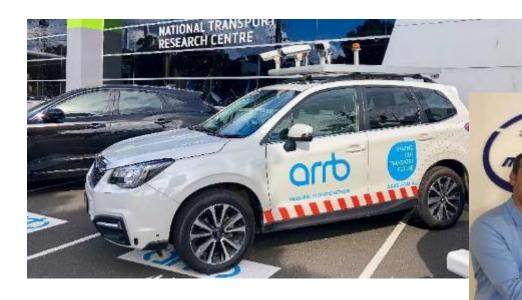
ARRB network survey vehicle with front facing cameras
